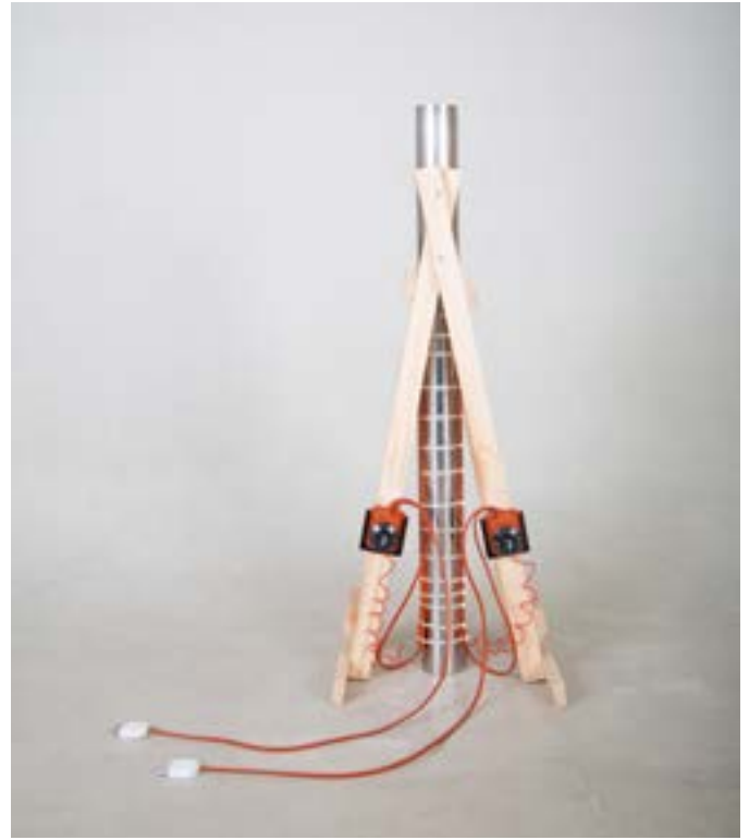
→ Plastification platform, used to soften wood and avoid fracture under pressure. Source: Vicente Carmona.
