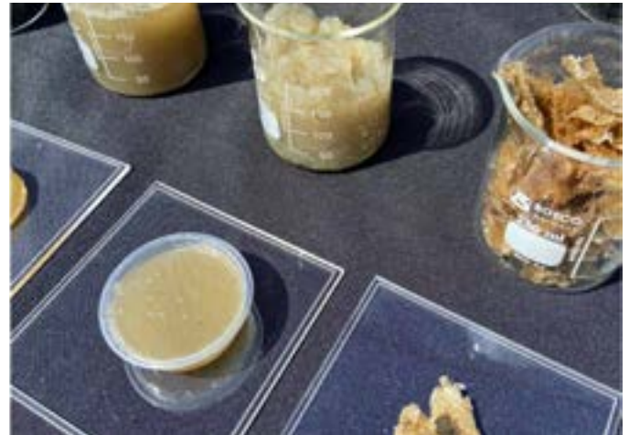
↑ Initial prototypes of bioplastic recipes based on Pelillo algae. Source: Tomás Vivanco.
