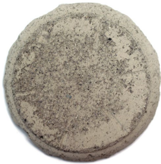
Experimento n°1: Concha de chorito (90%), cemento y yeso
